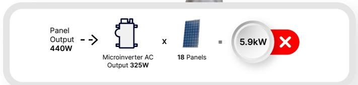
While the panel generates 440W of power, the microinverter only produces 325W, wasting the rest, resulting in a system that delivers less than what they expected.
